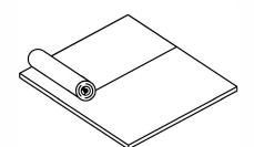
Install one roll of **Natura™** parallel to the wall and in the opposite direction as you plan to install the flooring planks, with the vapor barrier film (blue side) facing down.
