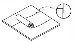
Cut the underlayment with a utility knife 1/2" to 3/4" away from the wall. Install the planks, but be sure that you are still able to see the edges of the underlayment so that you can properly line up the next roll.
